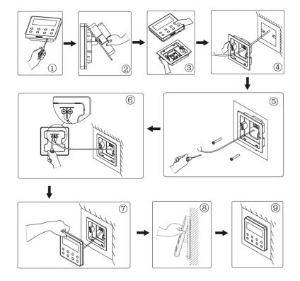
Figure 2-5-2 Installation of wired controller
