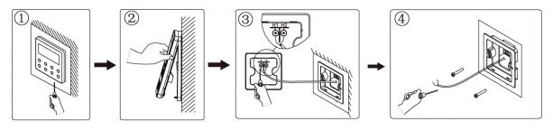
Figure 2-5-3 Removal of wired controller
